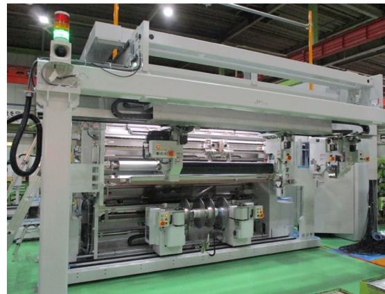
Film slitter for electronic component manufacture
