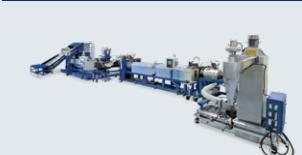
Integrates all processes, from crushing and melting waste plastic to producing pellets. The equipment is used to manufacture pellets that serve as raw material for recycled plastic.
